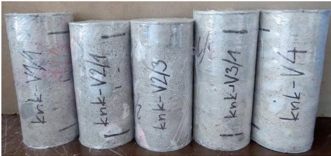
Fig. 8. The taken concrete specimens for dynamic and Young's modulus of elasticity and compressive strength testing in the laboratory
