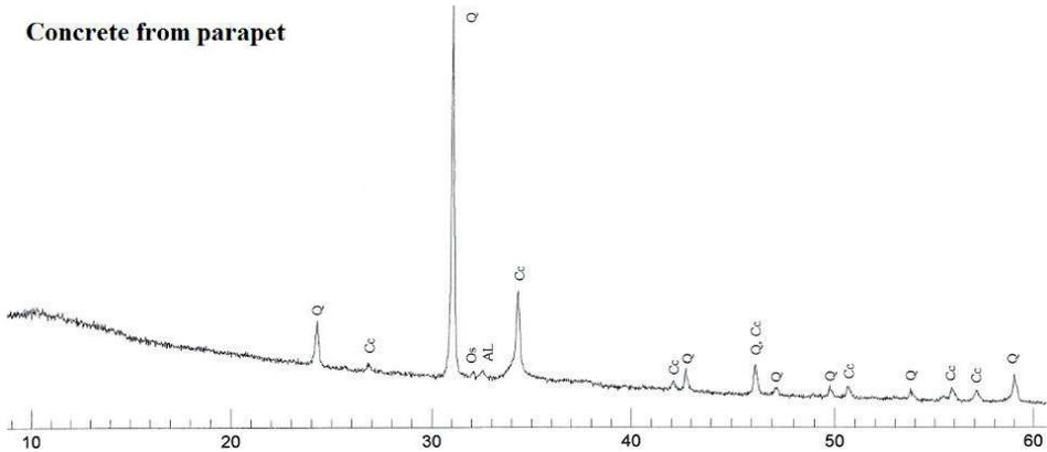
Fig. 10. X-ray diffraction analysis of concrete from parapet 2
