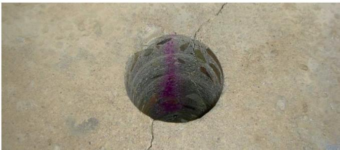
Fig. 6. Verification of carbonating concrete layer on the superstructure of the bridge
