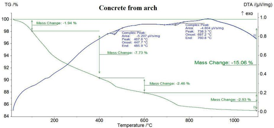
Fig. 11. Thermal analysis of the concrete from arch 2
