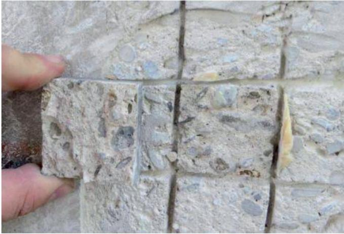
Fig. 5. Estimation of the adhesion – teared off surface concrete layer
