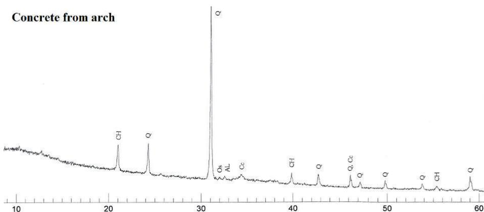
Fig. 9. X-ray diffraction analysis of concrete from arch 2
