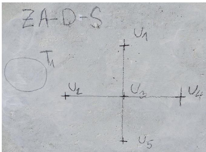
Fig. 4. Scheme of the transit time of ultrasonic wave measurement – test site ARCH1-U-C
