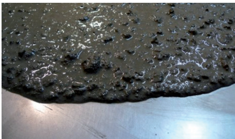
Figure 12. Fresh concrete appearance – Mix 2.
